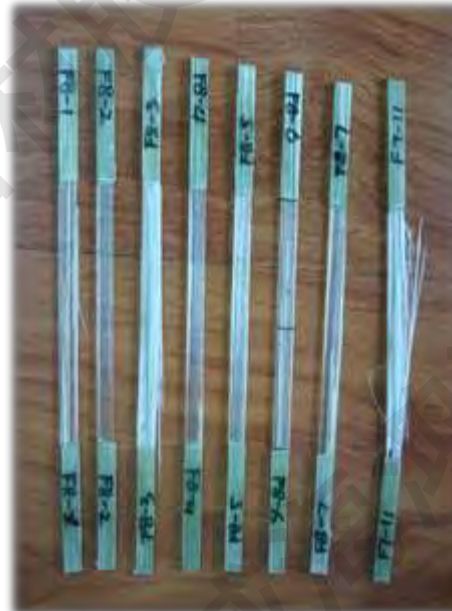
Specimen damaged after fatigue test
